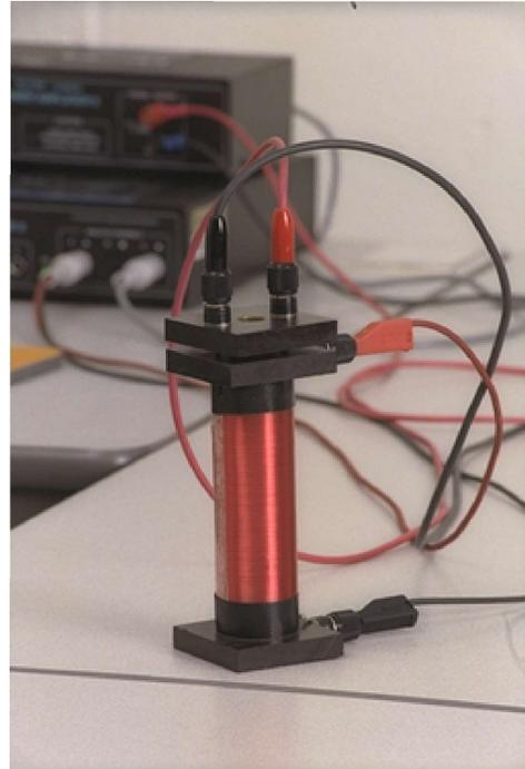
Now, you will need to hook up the smaller, primary coil to the “OUTPUT” terminals of the data interface as shown below.
